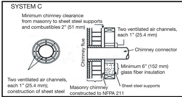
System C. Sheet steel chimney connector, minimum 24 gauge [0.024 in. (0.61 mm)] in thickness, with a ventilated thimble, minimum 24 gauge [0.024 in. (0.61 mm)] in thickness, having two 1 in. (25.4 mm) air channels, separated from combustibles by a minimum of 6 in. (152 mm) of glass fiber insulation. Opening shall be covered, and thimble supported with a sheet steel support, minimum 24 gauge [0.024 in. (0.61 mm)] in thickness.
